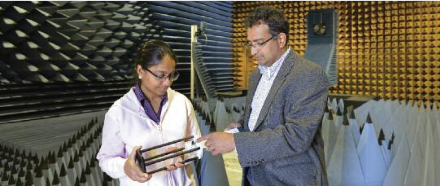
SUNY Oswego's anechoic chamber for development and testing of wireless devices. Credit: SUNY Oswego
