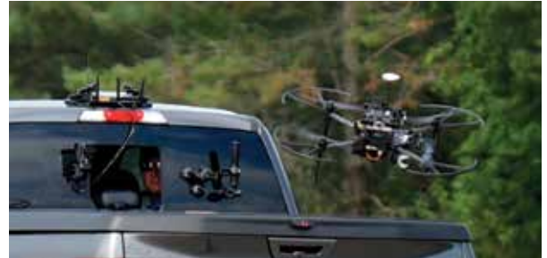
A DJI Matrice 100 autonomously launches from the bed of a moving Ford pickup truck on its way to a simulated disaster site during the 2016 Developer Challenge at Griffiss International Airport in Rome.
