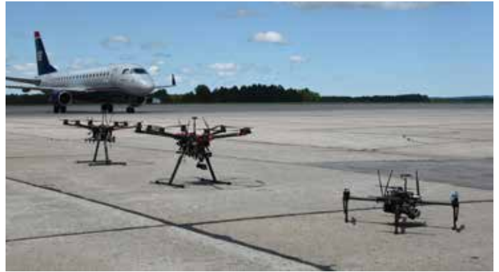
Pictured are three of the four unmanned aircraft (DJI M100 (closest), DJI S1000, DJI S900) that flew simultaneously for the NASA TCL2 tests. Flight data was sent in real-time to NASA as the aircraft performed different missions. Missing from photo is a fixed-wing FireFly6 Pro.
