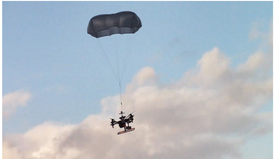
NUAIR recently validated the parachute system by Aerial Vehicle Safety Solutions (AVSS) by putting the drone it was attached to through 45 different failure scenarios.
